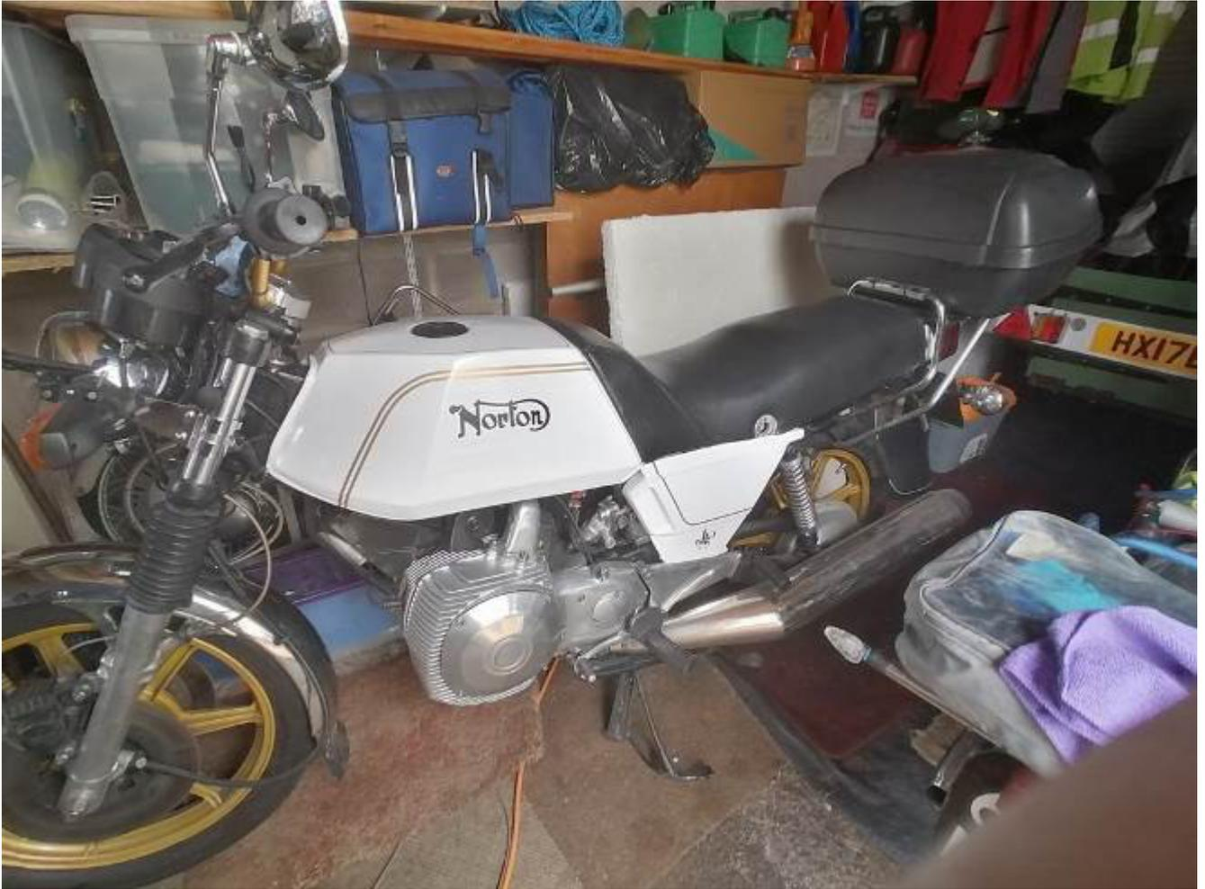
OR... White,1983 Interpol 2 , Rotary engine, Engine fully stripped, re-mollied, new bearings and seals, by George Molyneaux, bills to prove, new tyres last year, set of ASBO exhausts and loads of spares, carbs fully overhauled, ignition checked by manufacturer, forks by Marzocchi, Brembo brakes, Grimeca wheels as standard, powerful fast bike with electric start and excellent brakes, ready to ride in excellent condition, £6500ono, you won't find a better one,
