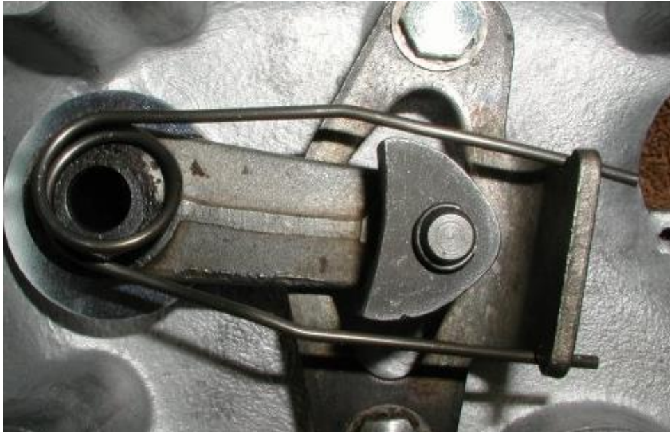
Incorrect ratchet spring fitment.
