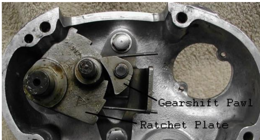
The ratchet assembly seen from the side.
