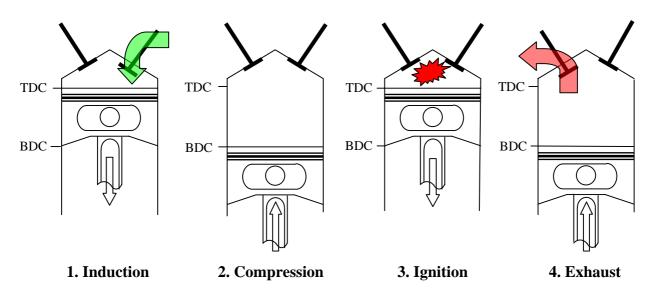
The diagrams above illustrate the conventional 4-stroke cycle of an internal combustion engine. It can be seen that both the intake and exhaust valves remain closed during the compression and ignition phases of the cycle. It is therefore usual for any discussion of valve timing to focus on parts 1&4 of the cycle, that is the valve motion in the periods either side of piston Top Dead Centre (TDC) on the non-firing stroke.
