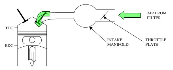
Whilst the engine is operating at full load, the throttle plate is turned so as not to restrict air flow into the intake manifold. The piston has only to draw air into the cylinder through the slight restriction of the air filter during the intake stroke and so the incoming air is at approximately atmospheric pressure.
