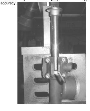
TAP M18X1.5 AGAIN THIS WILL NEED TO BE TAPPED TRUE TO THE BORE, I WOULD 3, RECOMMEND USING ONE OF THE PROPRIETARY TAP GUIDES OR STARTING THE THREAD USING THE DRILL PRESS AND THEN CAREFULLY CONTINUE IN THE NORMAL MANNER, WITH OUR TAP 8 ROTATIONS IS PLENTY (MINIMUM SEVEN ROTATIONS) AND THIS SHOULD GIVE THE 9MM OF FULL THREAD REQUIRED.
