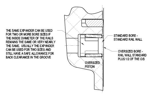
Hastings does use more than one rail with a given expander in many cases in order to build more than one ring set. For this reason and several others, the use of a flexible band to determine the suitability of an expander for a particular bore size is not practical.
