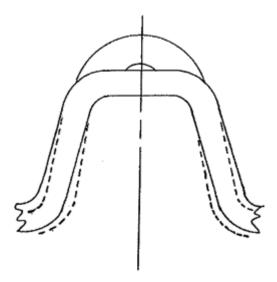
The solid line is the expander relaxed and the dotted line is the compressed state.
