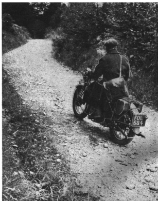
(Right) A restarting test on the 1 in 31 section of All-y-Bady, near Llangollen
